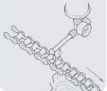
TYPE 2, Drip or Pressurised Lubrication
